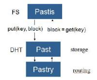
Security in the file system is achieved by signing a file inode before storing it in a PKB and by associating a CHB with a key obtained from hash functions. Modifying a file or directory in Pastis requires updating the PKB in which its inode is stored, but it is also involves the insertion of new CHBs reflecting the newly written data.
